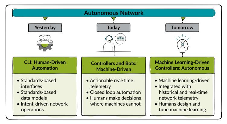
Autonomous network success depends on the performance of predictive algorithms, which depend on the data models (correlation engines). The fidelity of such data models is directly proportional to the amount of data collected (telemetry) from the network over time.
