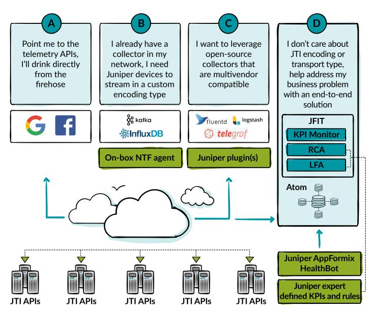
A key building block of a Self-Driving Network is automation equipped with real-time insight into all aspects of the network state, including device-level, service-level and component-level data. Telemetry is the enabler for 'closing the loop' and providing detailed instrumentation back to automation systems.
